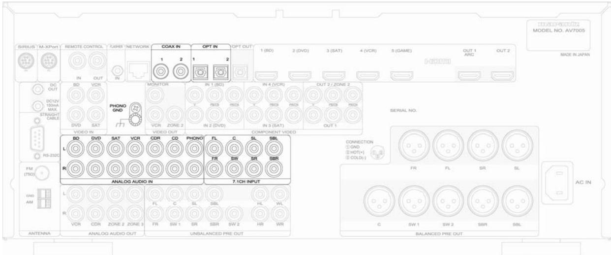
*Audio Input Connections (Digital and Analog)*
