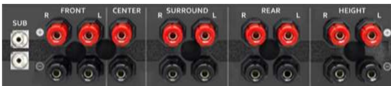
Figure 7: Rear panel of a 7.2.2 AVR; height speaker connections are at right.
