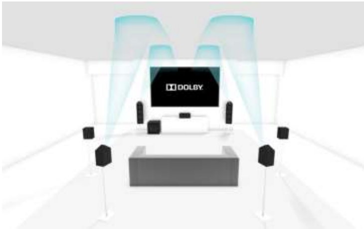
Figure 4: A traditional 7.1 speaker layout with four Dolby Atmos enabled speakers (7.1.4).
