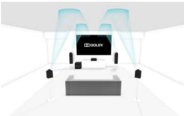
Figure 5: A traditional 5.1 speaker layout with four Dolby Atmos enabled speakers (5.1.4).
