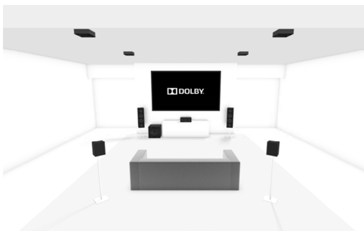
Figure 6: A traditional 5.1 speaker layout with four overhead speakers (5.1.4).
