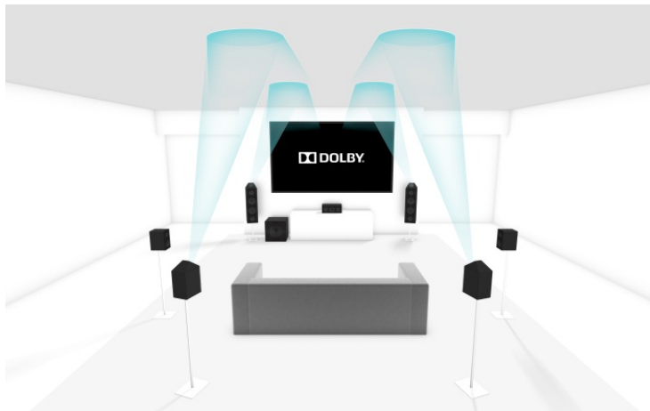
Figure 5: A traditional 7.1 speaker layout with four Dolby Atmos enabled speakers (7.1.4).
