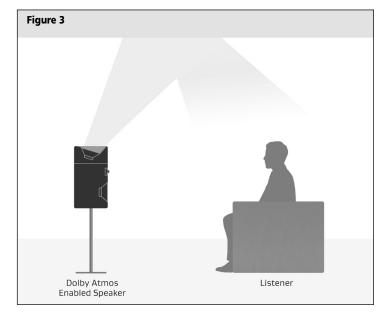
**VERY IMPORTANT:** The 44-DA speaker projects its sound from the top of the cabinet, not from the front like a conventional speaker. Do not place anything on the cloth grille on the top of the speaker, place the speaker in a cabinet or below a shelf. These situations will obstruct the sound path, impairing the performance, and possibly damaging the speaker elements beneath the cloth.
